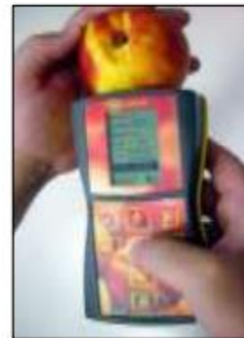
DA meter for non-invasive quality evaluation
