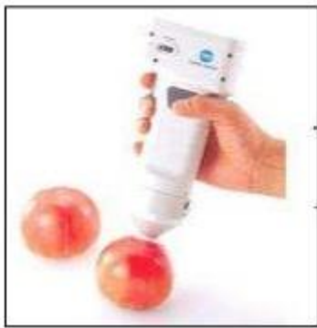
Colorimeter to quantify color
